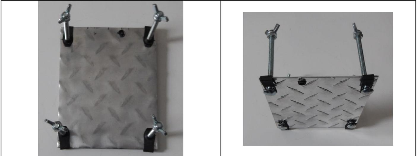
The pictures above show the top (left) and the bottom (right) of a Thin Panel Diamond Plate Aluminum Smart-D-Scope. Hardboard 1/8" thick as well as other thin rigid thin sheet materials can be used. Note that the clips are installed with the threaded portion on top. This allows for a greater range for focus adjustment than if the threaded portion was placed face down.
