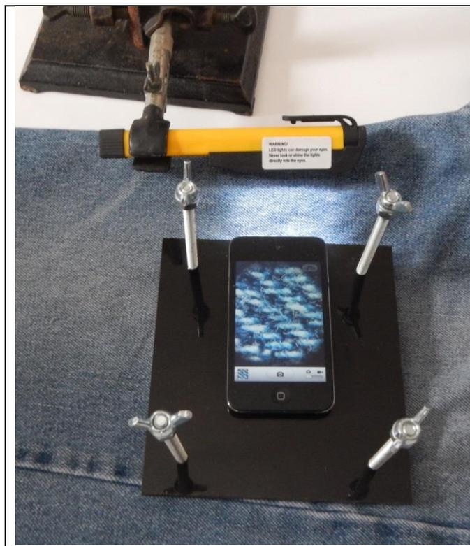
The image on the left shows a “Larry” LED flashlight held in a lab stand by a test tube clamp. The flashlight is illuminating the denim jeans. The image on the iPod shows the threads of the fabric. The stressed threads show the white inner core of the thread.
